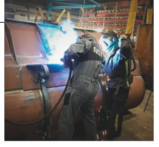
The flux cored wires in ICF may contribute to the increase of the welding works quality as they meet high requirements demanded by the welded constructions. The basic quality areas include the compliance with the low hydrogen process and acquisition of the technological weldability, complete identification and repeatability of the mechanical properties and high operational properties. They are also easy to store.
